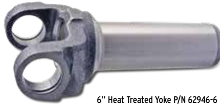
6" Heat Treated Yoke P/N 62946-6 1310-series 20° angle, 27-spline, 1 1/16" bridge Option 80119-6
