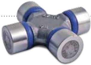
P/N 65382 • 1310-series, caps with grease fittings 1 1/16" Journal Assembly, 3 7/32" across bridge
