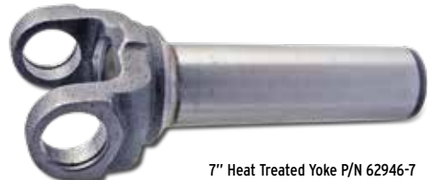
7" Heat Treated Yoke P/N 62946-7 1310-series 20° angle, 27-spline, 1 1/16" bridge Option 80119-7
