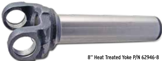
8" Heat Treated Yoke P/N 62946-8 1310-series 20° angle, 27-spline, 1 1/16" bridge Option 80119-8
