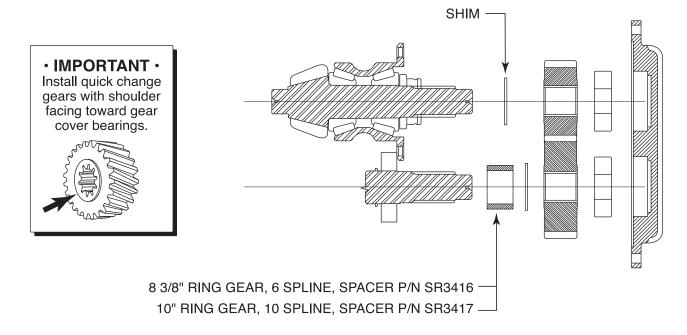
Helical Gear Spacer Kit P/N SR3551 (for 6 spline)
