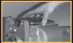
1. Install both detent balls and springs into 2. Side cover installation. Make sure gasket is in place and detent springs and balls are in their proper places. Torque side plate bolts to 15 ft lbs.
