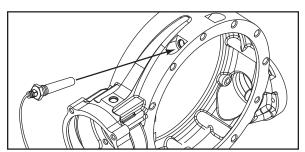
Illustration shows location of the breather assembly when installed.
