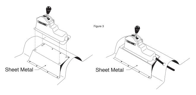
Illustrated above is a suggestion for tunnel-mount applications of the Winters shifter. By bending a piece of sheet metal suitable for your particular application, a flat surface will be obtained allowing your shifter to be securely fastened in the proper location. Make sure the sheet metal is of substantial gage thickness (18 or 20 ga.) or securely braced to minimize undesirable vibration.
