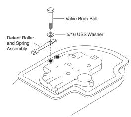
The shift feel of the Turbo-Hydro '400' transmission can be greatly enhanced by placing a 5/16" USS washer between the valve body bolt and detent roller and spring assembly. To gain access to this bolt the transmission fluid must be drained and the pan removed. Please consult proper service manual for removal instructions.
