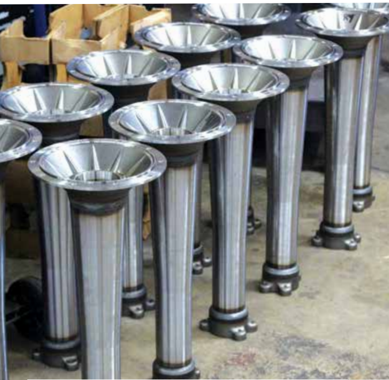
Tapered steel tubes and bells have been welded and are on their way to be mated with their center sections in the assembly department.
