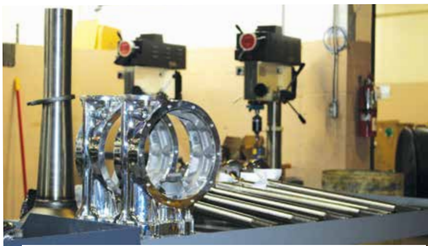
Quick changes are available in natural cast or polished finishes. Here a cart of polished center sections, tapered steel tubes and bells, and axles await final assembly.
