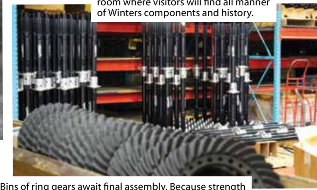
Bins of ring gears await final assembly. Because strength is a priority, Winters uses ARP ring gear bolts exclusively.
