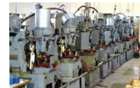
While hobbing machines handle parts like spur gears, these shapers are used for internal and external splines on tubes and shafts.
