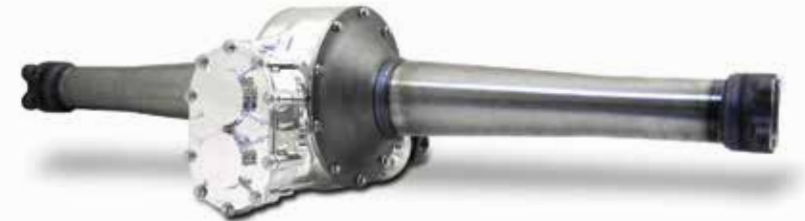
Perhaps the most popular rear among hot rodders is the Steel Tube and Bell V8 Quick Change. It features an 8-3/8" 3.78 ring and pinion, Winters Wedglock differential, 6-spline spur gears in the customer's choice of ratio, and original Ford-style tapered steel tubes and bells. V8 Quick Changes are rated up to about 600 horsepower.
