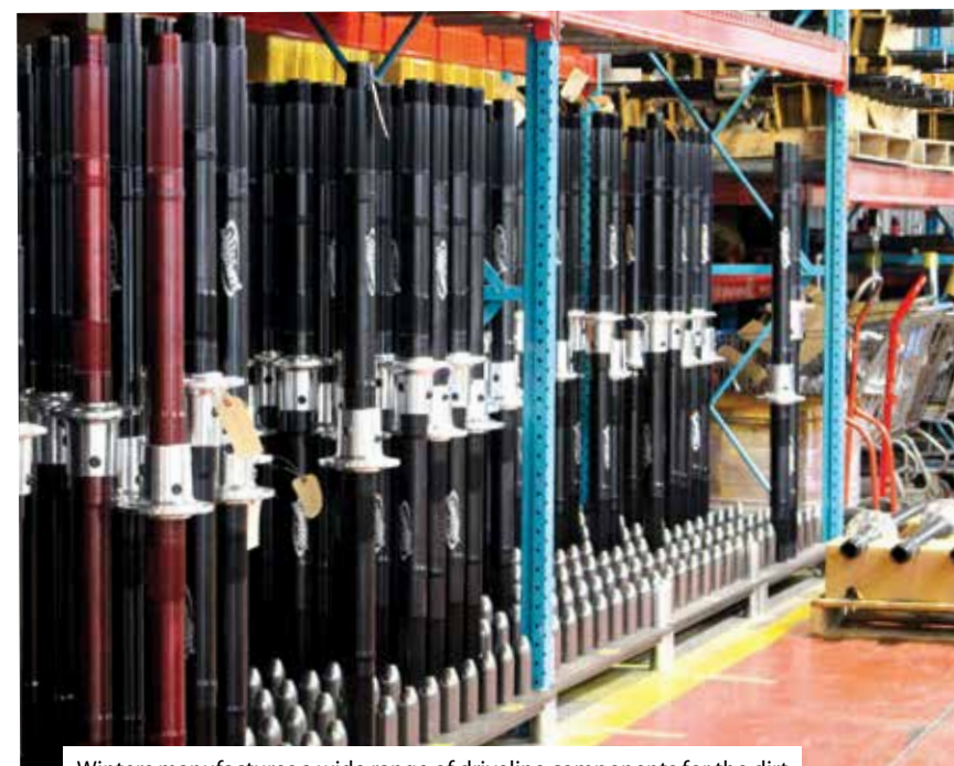
Winters manufactures a wide range of driveline components for the dirt and asphalt racing world. These are pallets of live axles for Sprint cars.
