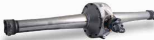
These brand new Banjo rears replicate the OE banjo look but with modern ring and pinion, differential and internals. They are available in both V8 and Champ sizes with steel tubes and bells or ribbed bells with straight tubes.
