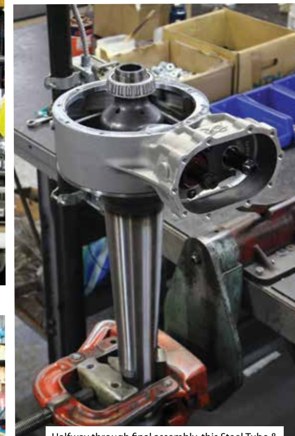
Halfway through final assembly, this Steel Tube & Bell V8 Quick Change already has its Wedgelock differential and bearing cone installed.
