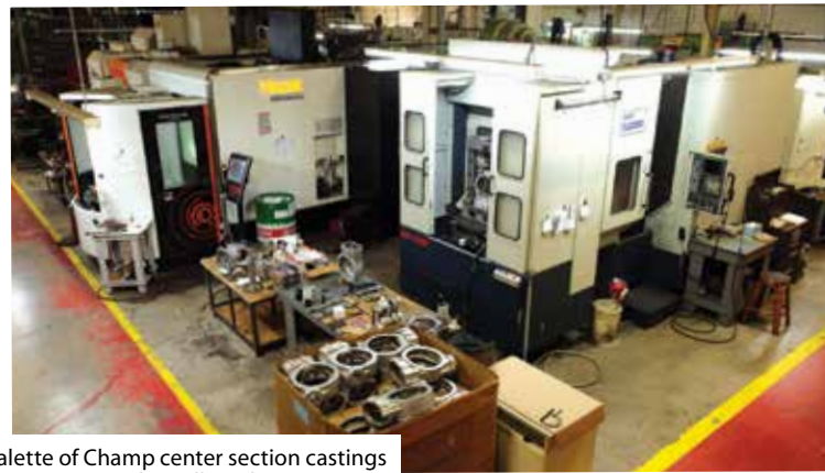
A palette of Champ center section castings awaits its turn in the milling department.
