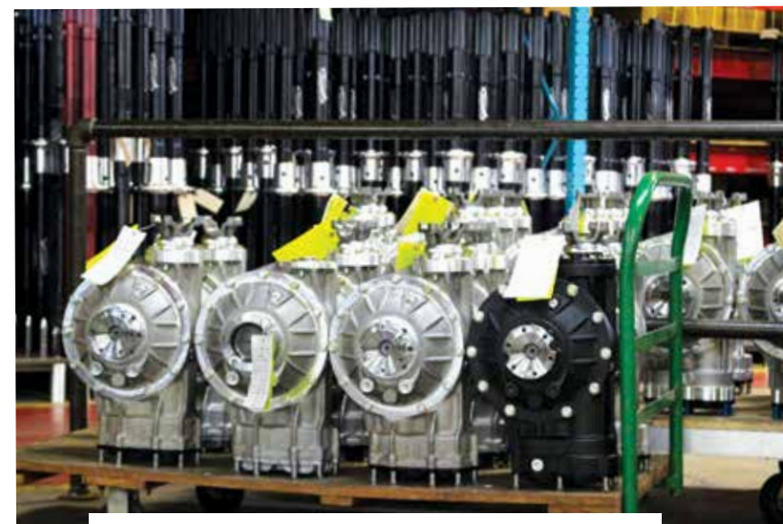
Completed Independent Quick Changes in natural cast and thermal dispersant-coated finishes are bound for the shipping department.
