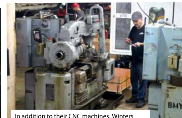
In addition to their CNC machines, Winters employs a great deal of manual equipment like these hobbing machines for cutting splines in shafts and performing other operations.
