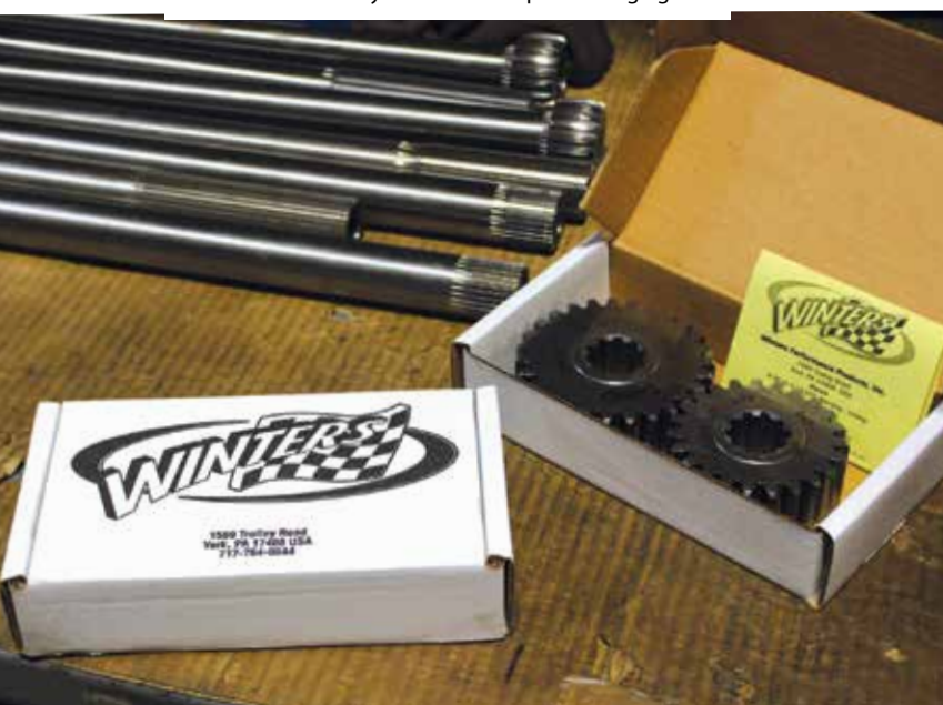
Winters offers nearly 100 gear sets collectively for their quick change rears—which equates to nearly 200 available ratios.
