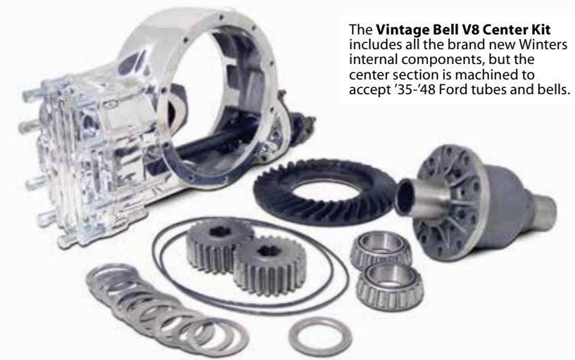
These brand new Banjo rears replicate the OE banjo look but with modern ring and pinion, differential and internals. They are available in both V8 and Champ sizes with steel tubes and bells or ribbed bells with straight tubes.
