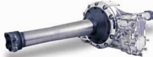
The Champ Quick Change features a 10" 4.12 ring and pinion, Winters Track differential and customer's choice of 10-spline spur gear ratio. Shown here is the Champ Adapter, which allows for the use of either Winters' V8-style tubes and bells or original '35-'48 Ford tubes and bells. Champ Quick Changes are rated to about 1,000 horsepower.
