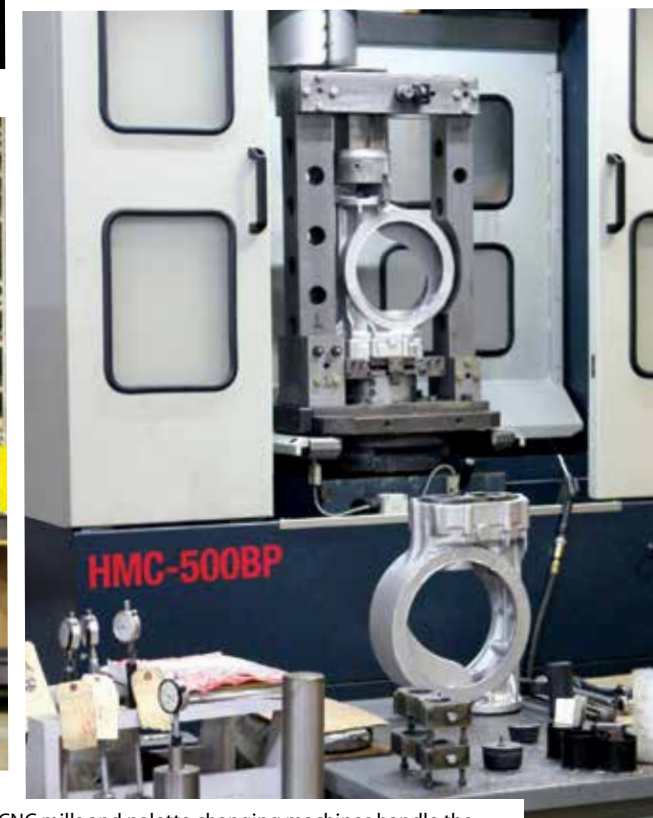
CNC mills and palette changing machines handle the operations necessary to take a raw center section casting to a finished piece. This first operation machines the face and interior, then drills and taps the holes to mount the bells. A five-axis mill handles the rest of the machining.
