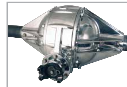
Assembly P/N SR3920 shown with 1350-Series Yoke (Option SR8275-1) Polished Finish (Option SR8207-308)
