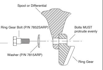
Caution: When using a steel spool, ring gear bolt must be shortened to allow for clearance between bolt end and center housing.
