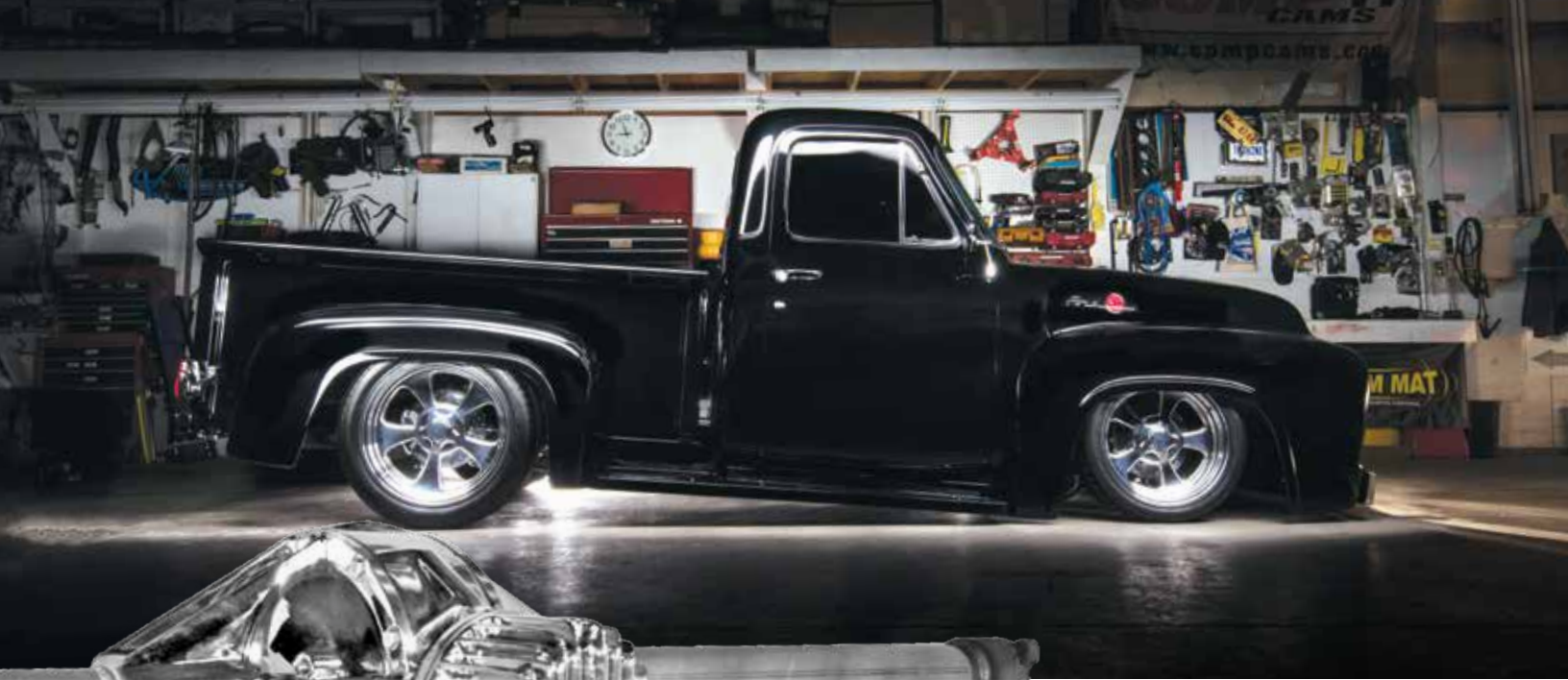
Champ Heavy Duty Quick Change rear in Classic Restorations of Southern Indiana's 1955 Ford F-100. The Champ HD features the same 10" 4.12 ring & pinion that's in all Champ Quick Changes, but with a reinforced center section and deep dish gear cover designed for higher horsepower applications. Photo by John Jackson/NotStockPhotography
