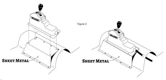
Illustrated above is a suggestion for tunnel-mount applications of the Winters shifter. By bending a piece of sheet metal suitable for your particular application, a flat surface will be obtained allowing your shifter to be securely fastened in the proper location. Make sure the sheet metal is of substantial gage thickness (18 or 20 ga.) or securely braced to minimize undesirable vibration.
