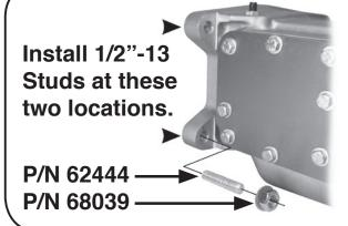
Install 1/2" - 13 x 2 1/2" studs and nuts to retain transmission to flywheel housing on left side (optional at four locations).
